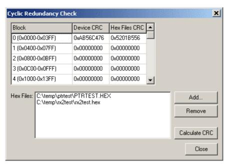
When the window is first opened the CRC value is read from the device for each Flash Block and the entire device. These values are shown in the "Device CRC" column.
