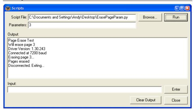
Choose the script file to run by clicking on the Browse... button. Enter any necessary parameters into the Parameters box and click on Run. The script can be stopped at any time by clicking on the Stop button.
