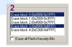
Select each Flash block that you wish to erase by clicking on its name. If you wish to erase all the Flash then check that option. If you check to erase a Flash block and all the Flash then the Flash block will not be individually erased. If you wish to erase only the Flash blocks used by the hex file you are going to select, then check that option.
