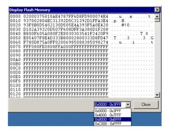
Each line shows 16 bytes of data starting at the address given at the start of the line. If a line contains question marks then data has not yet been read in for those locations. The memory is read in in the background allowing viewing of the memory that has been loaded in without having to wait for all of it to be read.
