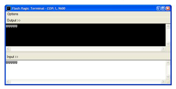
The top part of the window shows the output from the device. The bottom part is where characters are entered for transmission. The sizes of the areas may be adjusted by resizing the window and dragging the splitter located between the output and input areas.
