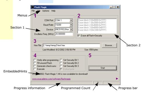
The window is divided up into five sections. Work your way from section 1 to section 5 to program a device using the most common functions. Each section is described in detail in the following sections.
