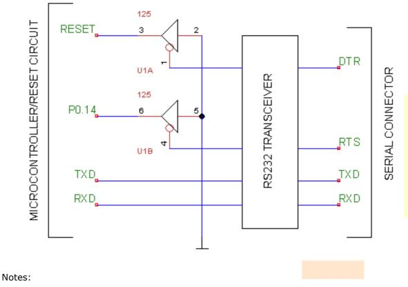
When the COM Port is not in use or the serial cable is not connected, the RS232 signals are pulled low by the transceiver. This results in the TTL signals being high. Therefore when the TTL DTR and RTS signals are high, P0.14 and RST must be in a state that allows the device to reset normally and execute code.
