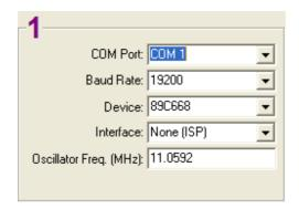
Select the desired COM port from the drop down list or type the desired COM port directly into the box. If you enter the COM port yourself then you must enter it in one of the following formats:
