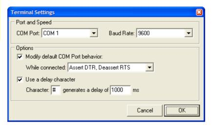
The default setting when the COM port is opened for the terminal interface, is that DTR and RTS are both asserted. This is standard COM port behavior. Because sometimes target hardware requires certain states for DTR and RTS it is possible to configure the state they will be in while the COM port is opened.
